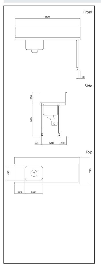
Handling System for Hood type Pre-wash Table with 500x400 Bowl and Strainer Right to Left, 1800mm
